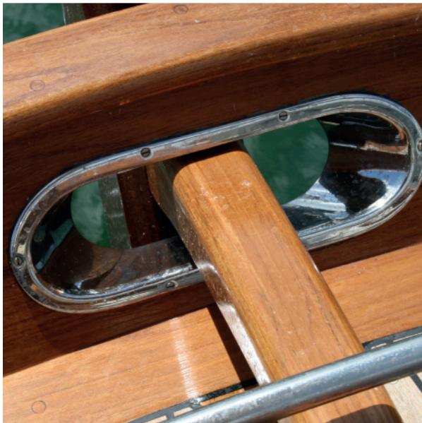
Clockwise from top left: bowsprit traveller and bronze furler; mainsheet block with its own cleat; gooseneck pin rails made by Peter; tiller aperture in the transom bulwark
